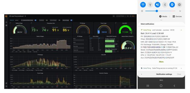
SolarThing allows you to monitor your battery voltage, incoming solar power, and power usage. Each datapoint can be graphed over time. Grafana allows you to view historical data and current data. SolarThing also supports 1-Wire temperature sensors, so you can record the indoor or outdoor temperatures. With more advanced configurations of SolarThing, it can be used as an automation system.
